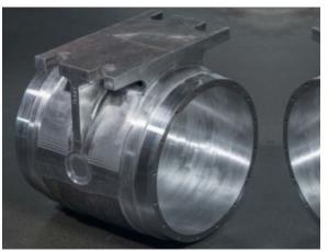
Pipeline's parts are made of steel - A350Gr.LF2, A420Gr.WPL6, A182Gr.F5, A234Gr.WP22, A182Gr.F321, A182Gr.F347, A403Gr.WP304 and other grades as agreed with the customer.
